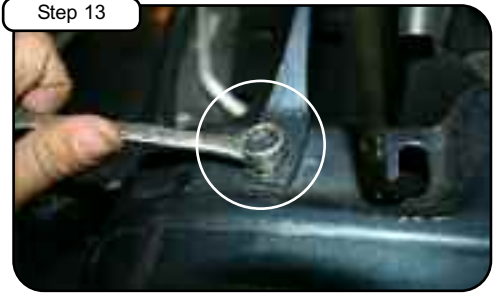
Step 13 Secure core support bracket using 13mm.
