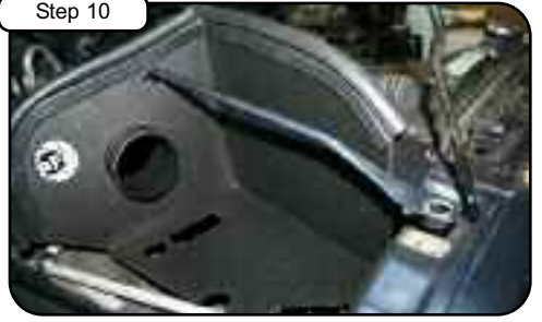
Step 10 Attach trim seal to housing and install. Make sure core support bracket slides through hole on housing.
