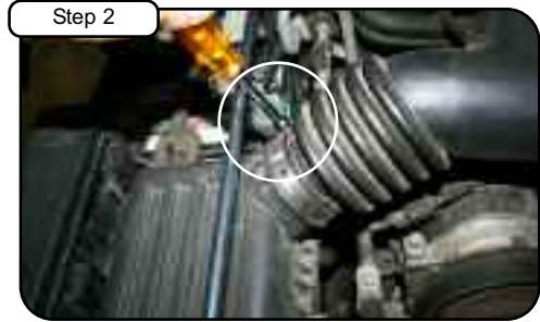
Step 2 Loosen clamp on stock intake using 5/16" nut driver.
