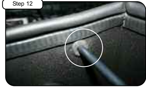
Step 12 Align grommet from step 8 and position in hole to prevent core support bracket from vibration.
