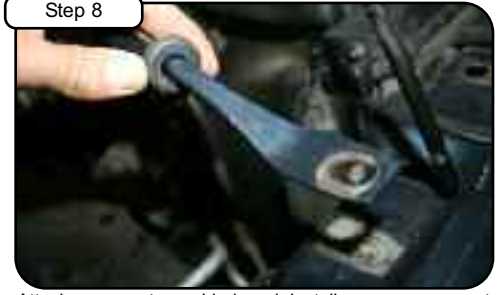
Step 8 Attach grommet provided and install on core support bracket.
