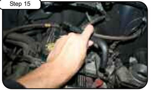
Step 15 Remove crank case line from engine.
