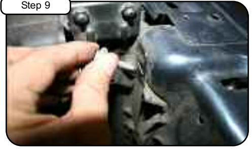
Step 9 Loosen bolt on core support using 10mm wrench. Save bolt for later install.
