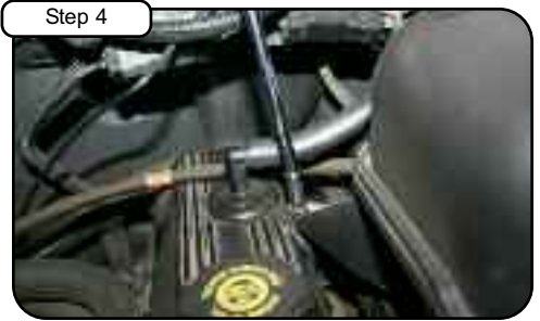
Step 4 Loosen bolts holding in stock intake tube on valve cover using 8mm socket or wrench and remove.
