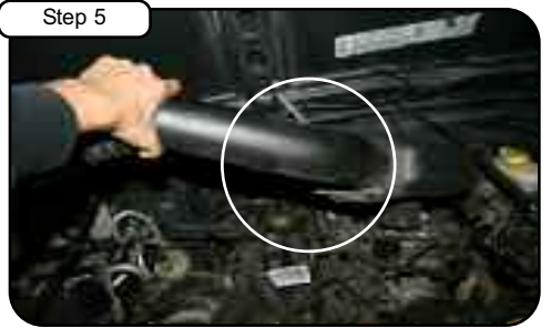
Step 5 Pull crank case line away from stock intake and remove from vehicle.
