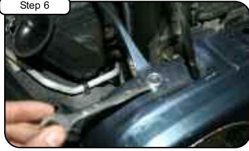
Step 6 Loosen bolt on core support bracket using 13mm socket or wrench.
