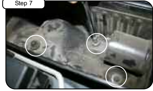
Step 7 Remove upper half of air box. Loosen the 3 bolts on bottom of air box using 8mm socket or wrench and remove.
