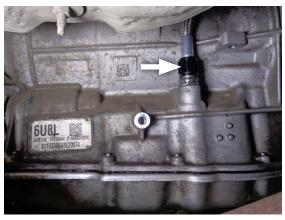
9. Push tube into fill port on passenger side of transmission until it's fully seated.
