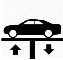
Note: Vehicle must be level for stability and to obtain an accurate fluid level.
