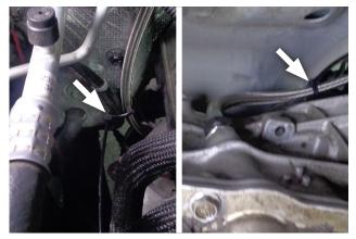
12. Use zip ties (x2) (1601022) to secure dipstick assembly. Make sure tube remains as straight as possible.
