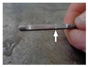
18. Once you have completed transmission fluid level check, remove dipstick and mark current fluid level on it. This will be your reference for future vehicle maintenance.
