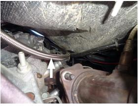
8. Find a suitable route for tube. Keep tube from touching exhaust components, as extreme heat can damage tube. Also keep tube from touching wires, brake lines, etc., as steel braid may cause chafing damage.
