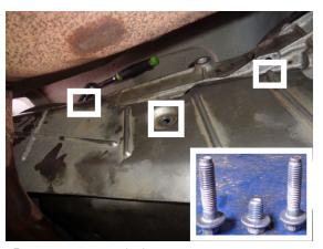
5. Remove bolts (x3) attaching cover to passenger side of transmission. Retain for later use.
