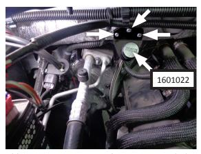
Install mount using Self Tapping Screws (x3) (3401568), checking for bindings in tube as each screw is fastened, then install dipstick (1601022) into tube and tighten it (until o-ring is compressed).
