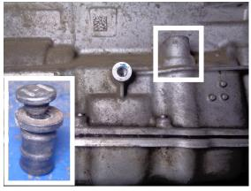
6. Release fill plug cap then remove it from passenger side of transmission.
