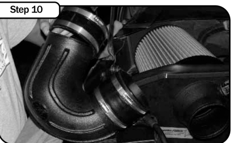
Place clamps and couplers provided onto new tube. (4 -1/2" coupler at filter side and 4" high temp at turbo side)
