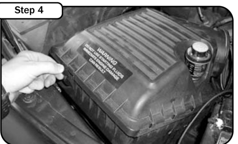
Release the 4 clips holding in upper OE air box and remove. ( Remove filter minder and grommet from air box and set aside for later install )
