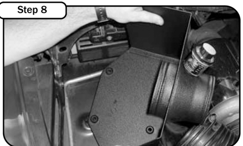
Install new housing into vehicle to OE position. Install 3/4" trim seal to housing.
