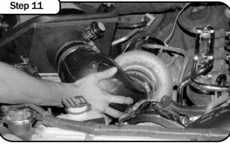
Install new tube and tighten using 5/16" nut driver.
