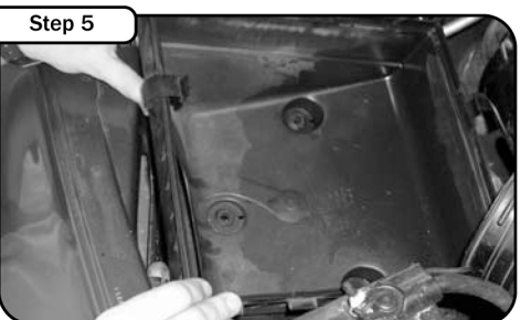
Carefully grab and pull out OE air box from vehicle.
