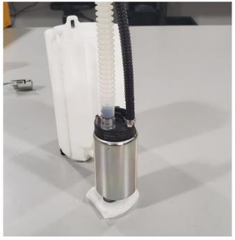
6 – Install the DW440 pump into the rubber bushing and plastic spacer, install the pump assembly into the bucket and click it into place. Be sure the pump is pushed all the way to the bottom of the bucket.
